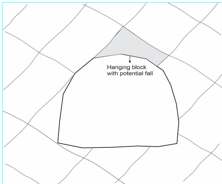
Figure 3. Potential block fall from the roof of an underground structure located at shallow overburden
