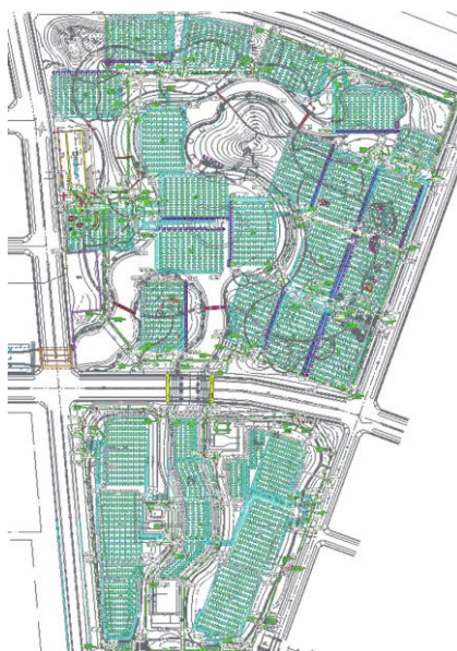
Figure 2. Schematic Diagram of Geothermal Borehole Layout at Beijing Daxing International Airport [35]
