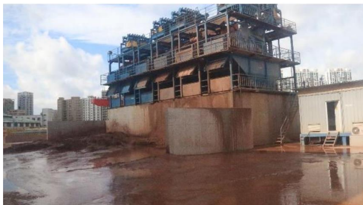
Figure 6. Slurry Separation during Construction Waste Processing for Shenzhen Metro Line 13 [45]
