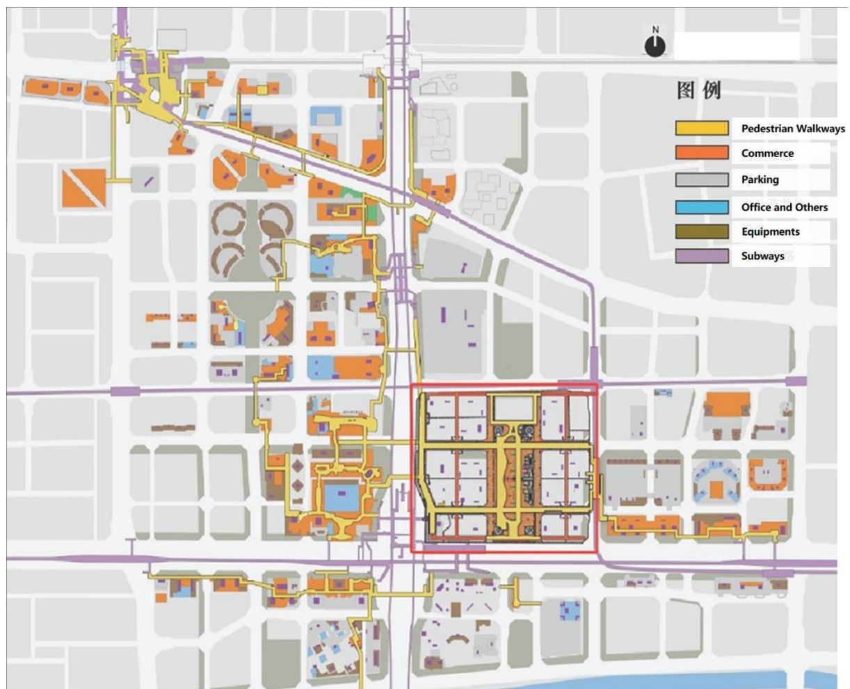
Figure 7. Schematic Planning Diagram of Underground Space System at B1 Level in CBD
